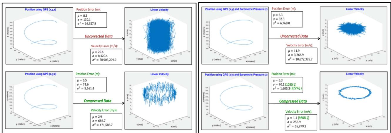
Figure 2. Comparison of GPS z vs Barometric Pressure z Error Correction
