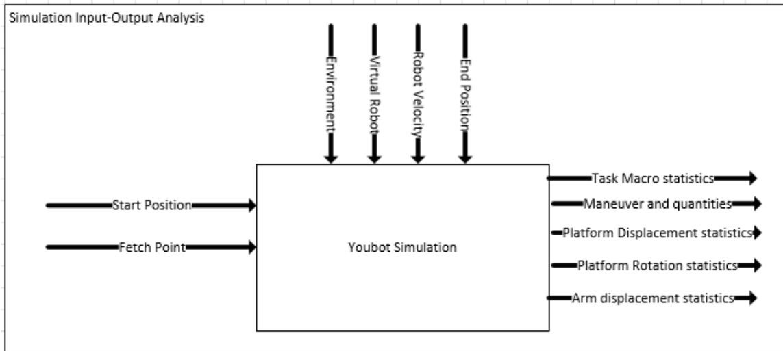
Figure 13 Input-Output Diagram
