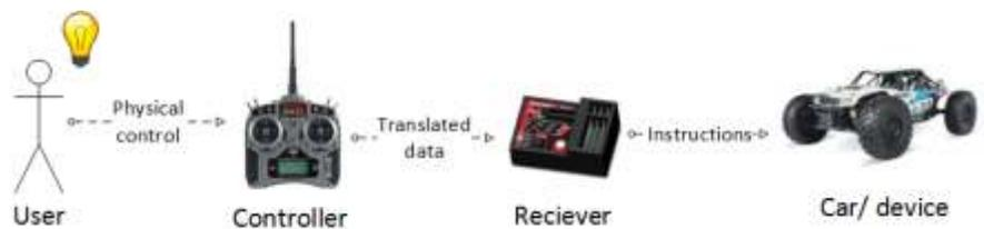
*Figure 1 HMI of an RC Car*
