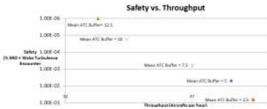
Fig. 7 Output from the ROQA simulation has similar results from earlier study showing reduction in safety with increasing throughput
