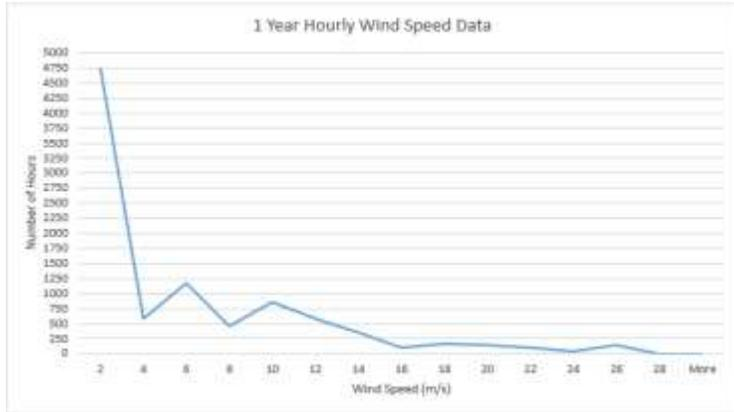
Fig. 7 hourly wind speed data over one year
