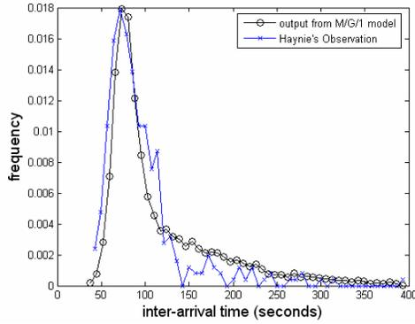
**Figure 5. Landing Time Intervals from a M/G/1 Simulation Model and Haynie's Observation**
