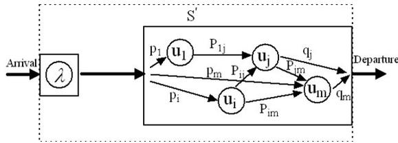
Figure 7. A Virtual Server with  $m+1$  Phases
