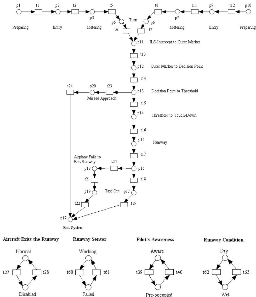
**Figure 5.** Petri net diagram of nontowered airport
