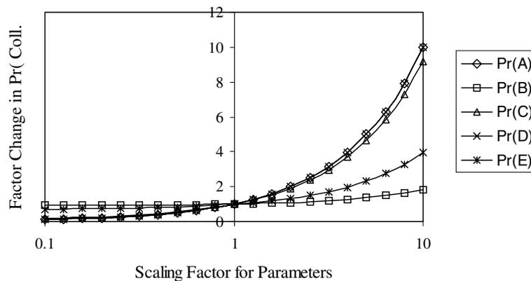
**Figure 8.** Sensitivity of collision probability to model parameters (the curves for Pr(A) and Pr(D) overlap)
