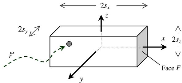
**Figure 1.** A geometric representation of the Reich collision model
