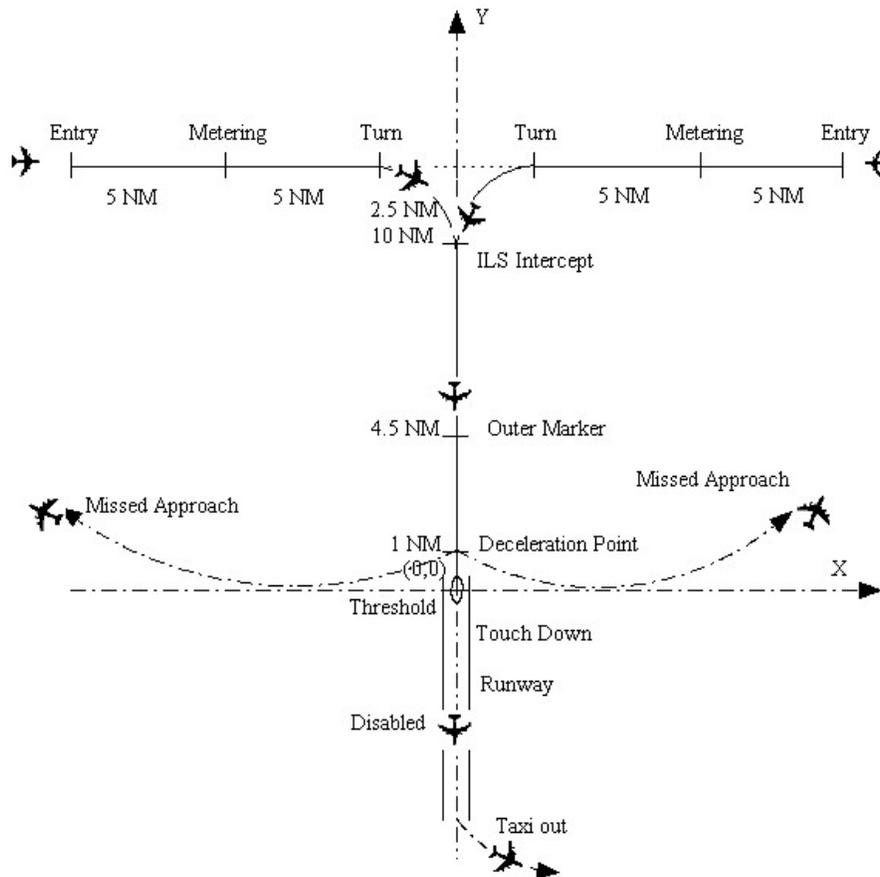
Figure 4. Airplanes landing at a small nontowered airport
