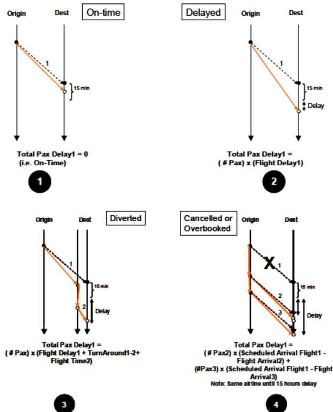
**Figure 1.** Passenger Trip Delay (solid) is determined by one of the scenarios described in Space-Time diagrams. The dashed line corresponds to the scheduled arrival time of the flight.
