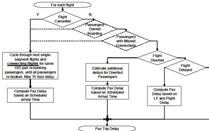
**Figure 2.** Algorithm used to compute Passenger Trip Delays. Dashed elements identify limitations of the algorithm that are under development.
