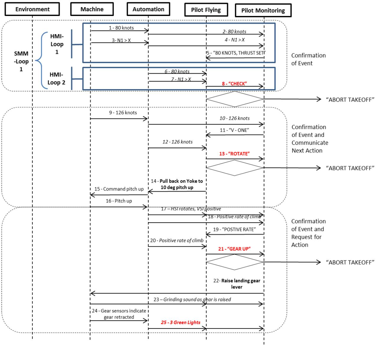
Figure 4 HMI-SD for a portion of the takeoff roll procedure
