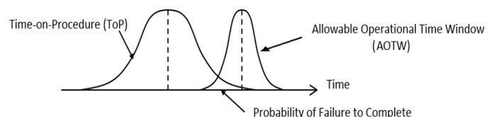
**Figure. 2.** Time-on-Procedure (ToP) relative to the Allowable Operational Time Window (AOTW). When the ToP is longer than the AOTW (i.e. overlapping region), the procedure cannot be completed in the required time frame and the procedure is considered to be incomplete. The probability of occurrence is key performance metric
