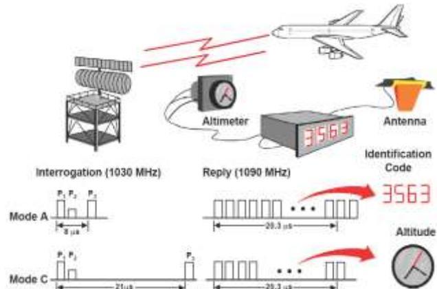
Figure 1: ATCRBS system working. Ref: Surveillance Tools for Distributed Air/Ground Traffic Management (Steven R. Bussolari, MIT, Lincoln Labs)
