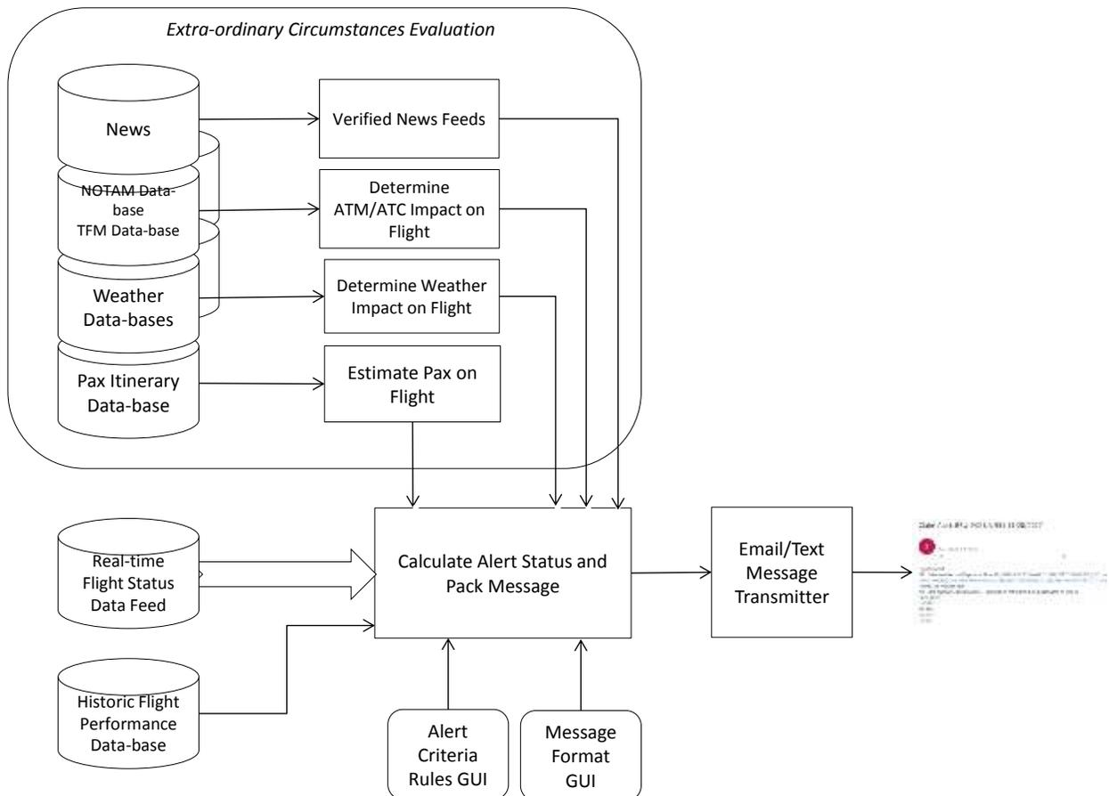
**FIGURE 1: System Architecture for Real-time Flight Status Alerting System (RtFSAS).**
