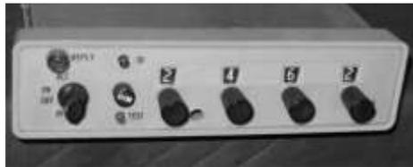
**Figure 1: A typical ATCRBS transponder (located in cockpit)**
